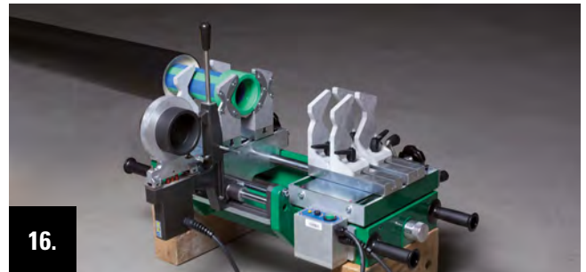
16. After the cooling time release the clamping jaws at the fitting and at the pipe end and turn the welding machine by 180°.
