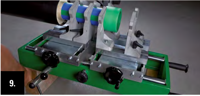
9. Drive the welding machine slide with the crank handle together and press the pipe end against the welding socket.
