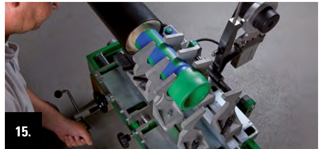
15. Drive together the welding machine slide with the crank handle up to the stop.
