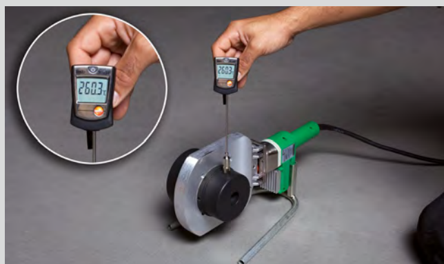
Measurement of temperature at the aquatherm manual welding device (1400 W )
