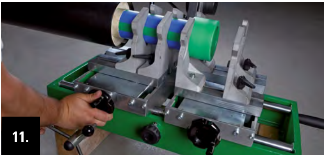
11. Fix the pipe end with the clamping jaws by turning the crank handle.
