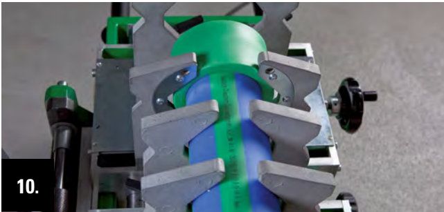
10. Align the pipe end circumferentially at the welding socket and center the position exactly.
