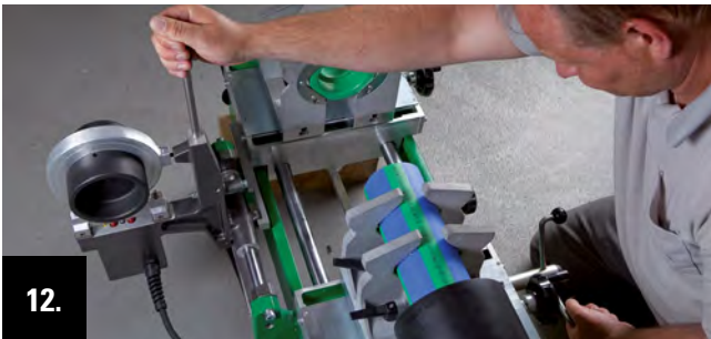
12. Drive apart the slide of the welding machine with the crank handle and pull out the calibration button for adjusting the welding depth.
