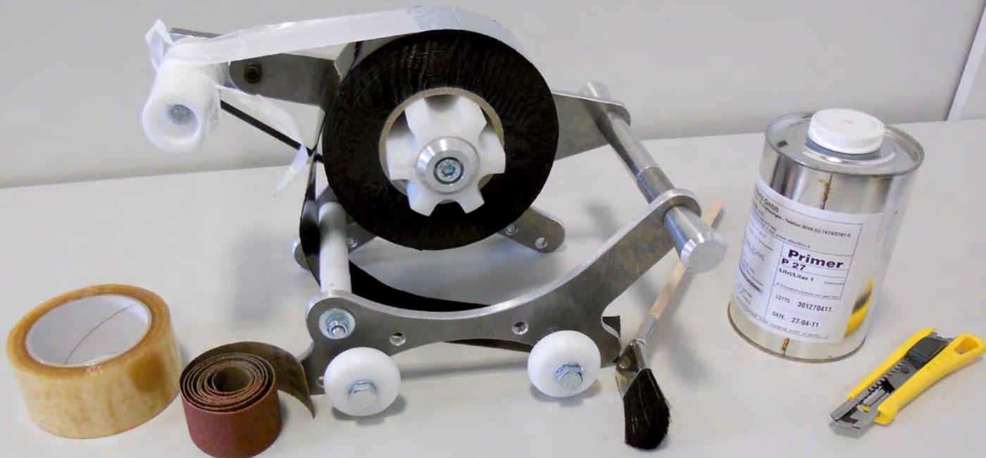
The winder shown below is not necessarily required for the processing of the MONO TOP 40 corrosion protective tape.
